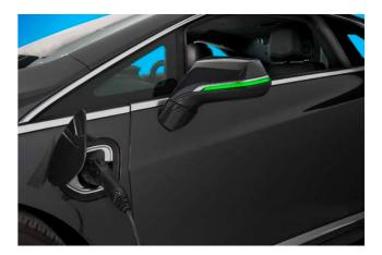
**Note:** Immediately after plugging in, the Charging Status Indicator on the instrument panel may be yellow for a few seconds before turning green. The charging system may run fans and pumps when the vehicle is turned off.
